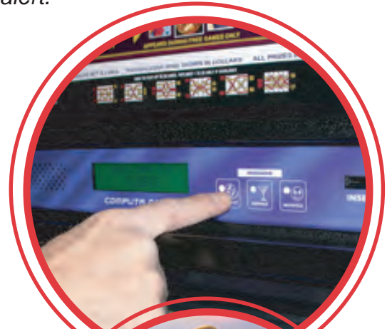
The paging request is received by the Loyalty System PC and sent to the Powerpage Transmitter
